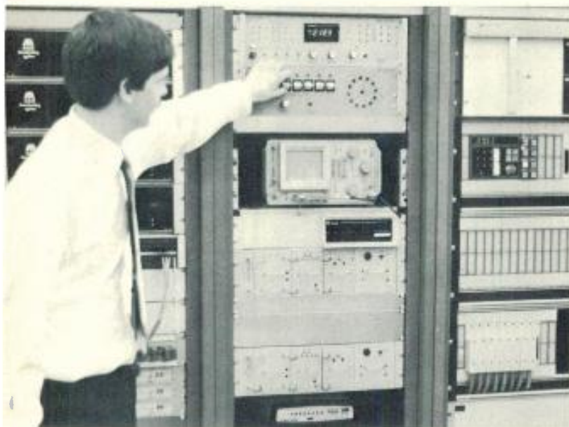
William Check, director of satellite engineering, demonstrates the modulator assignment control in the uplink electronics. Just below it is the spectrum analyzer that monitors output power
